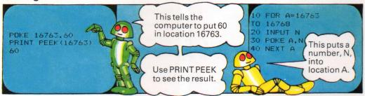
The picture above shows you how to use POKE. You can poke anywhere in RAM, but if you poke new values into the area reserved for use by the operating system you may disrupt the workings of the computer. You can restore it to normal by switching off and on again. Try writing a
